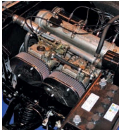
In a lightened Herald, this spec FWB engine should deliver as much as 150bhp per ton.
