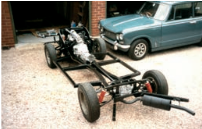
The Herald chassis was restored and modified with a bespoke rear end suspension of my design, turned into reality by Mike Brotherhood.
